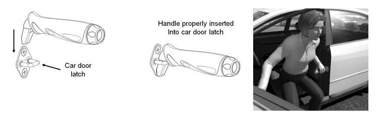
**IMPORTANT:** Do not attempt to insert the support handle into the car door latch in any other direction other than as shown in the above pictures. Failure to do so may cause injury and could possibly damage your car door latch. THE FLASHLIGHT SHOULD POINT TOWARD THE FRONT OF YOU CAR.
