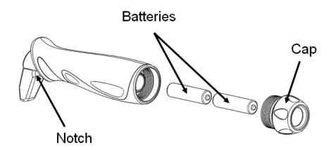
3. Replace the support handle cap by screwing the cap in a clockwise direction.
